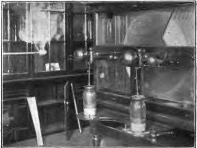
SMOKE FROM BURNING CAMPHOR, ON END OF GLASS TUBE, ASCENDS WHEN ELECTRIC MACHINE IS NOT IN OPERATION.
