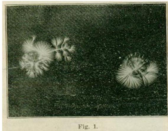
A one-inch spark from the small charging plates of the static machine produces a small electrograph as shown in Fig. 1. A 5-inch spark produces a larger electrograph, as shown in Fig. 2, and a 10-inch spark produces an electrograph still larger, as shown in Fig. 3. That is, the area of the electrograph increases with the potential.
