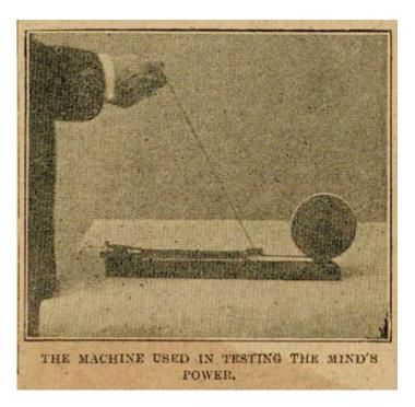
The instrument is known as the myergesthesiometer—truly an up-to-date scientific title. The pupil takes hold of the handle and rapidly pulls the cord, which unwinds from the pulley, as may be seen in our illustration. By an ingenious mechanical device the pull requires a uniform amount of energy throughout the whole length of the motion.
