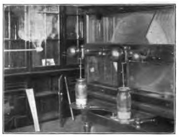
SMOKE FROM BURNING CAMPHOR, ON END OF GLASS TUBE, ASCENDS WHEN ELECTRIC MACHINE IS NOT IN OPERATION.
